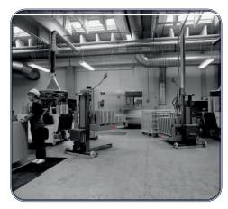
Translyft pallet lifters are ideal for use in compensation for differences in work levels, in particular when used with palletised loads.
